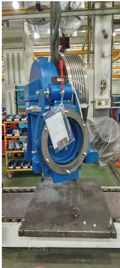
Figure 4 TGD3 Machine Recommended Hoisting Without Motor
