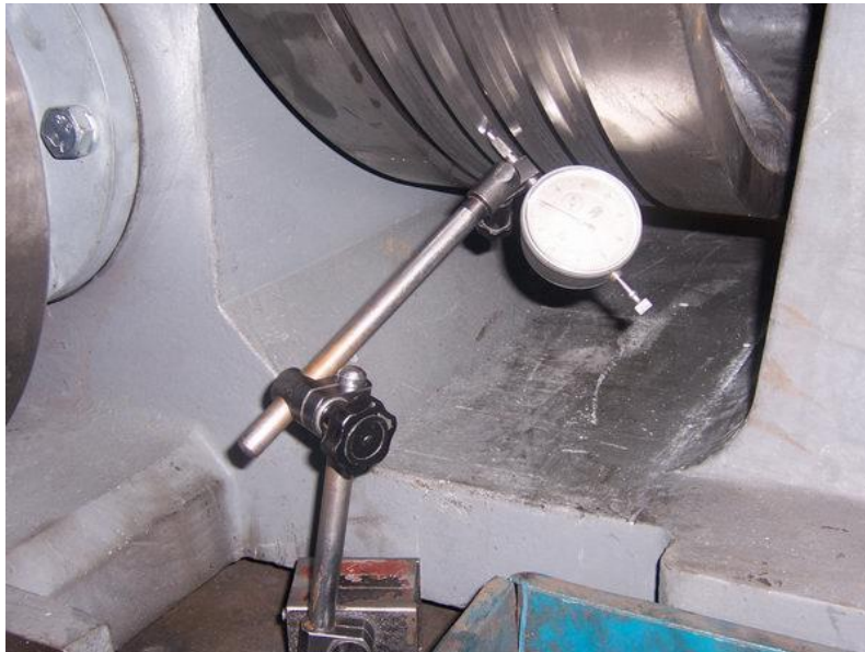
Figure 30 Dial Indicator position
