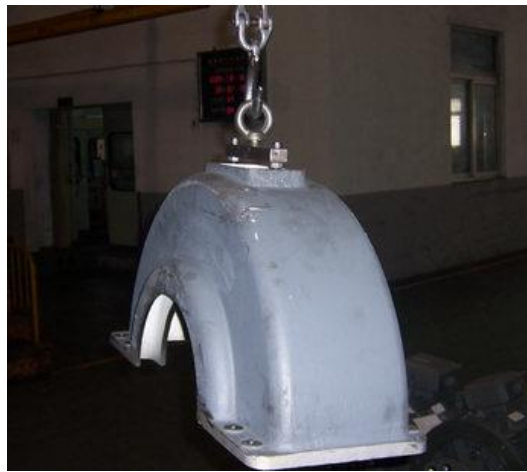
Figure 22 Hoisting the Gear case top
