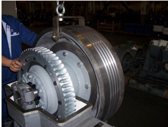
Figure 24 Sling the sheave and gear
