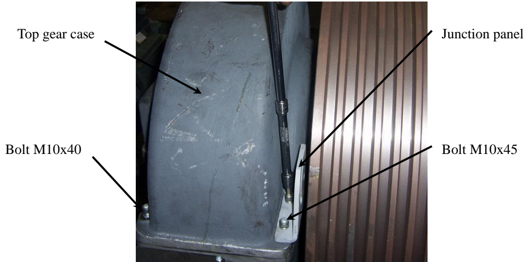
Figure 20 Junction panel removal
