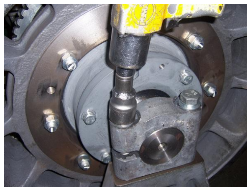
Figure 23 Remove the Support Body bolts.
