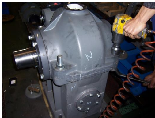
Figure 53 Gear Case Top reinstallation
