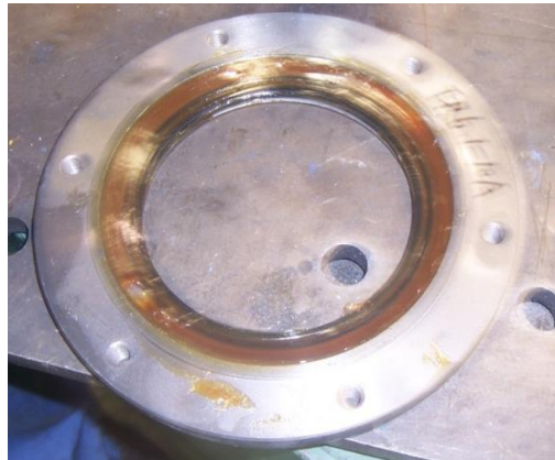
Figure 87: Apply grease to Outer cover
