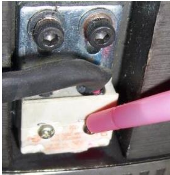
Figure 28: Apply Loctite 243 or equivalent
