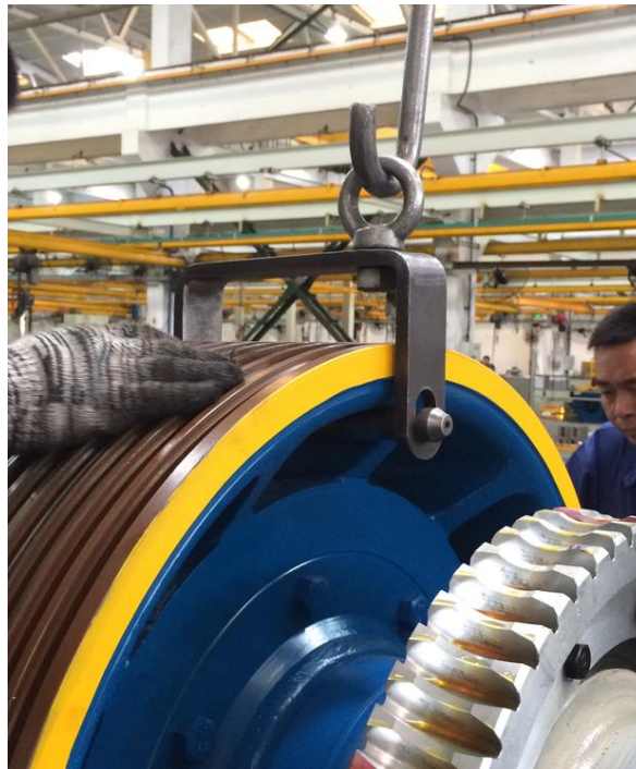
Figure 26 Sling the sheave and gear
