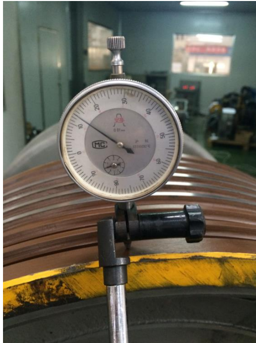
Figure 32 Dial Indicator position
