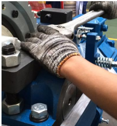
Figure 35 Tighten the two bolts
